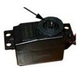
**9)** Put glue (\*) on the section of only one servo-motors (the section which is opposed to rotation axle - see photo).
