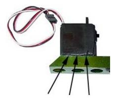
11) Let IMPERATIVELY dry the assembly during several hours so that good held mechanical (it is imperative to observe this condition to obtain a perfect assembly and not to be likely to put glue not perfectly dry on the fingers (\*)).
